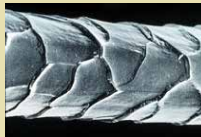
(Left) SEM (scanning electron microscopy) view of polymer coated wool fiber. Note scales on the merino fiber's surface (Right). SuperWash effectively reduces the scale's profile and the resin smoothes them over adding softness and abrasion resistance. Source: CSIRO, Canberra, Australia
