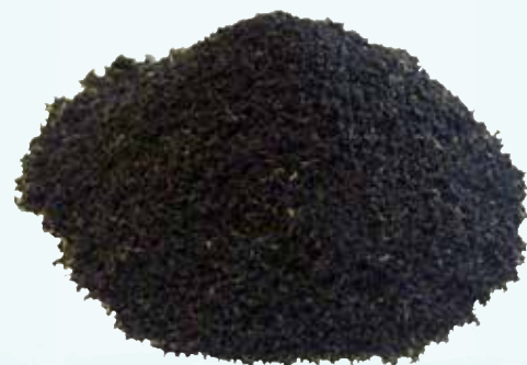
APX, 100% devulcanized rubber ready to be added or upcycled into a rubber master batch as virgin rubber (image courtesy of Tredagain).
