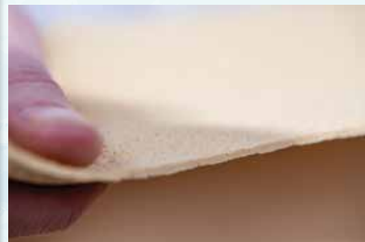
SolarCore polyfoam infused aerogel, cold rated to -58F or -50C
